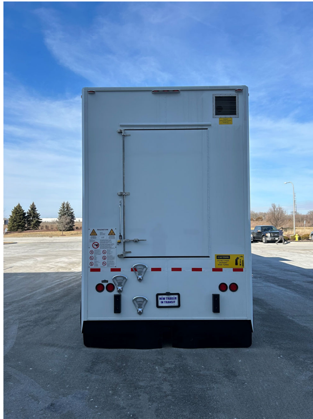
Figure 15: Magnet Room Helium Rear Door
