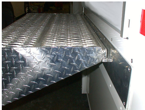
Figure 20: Stair Assembly (standard)
