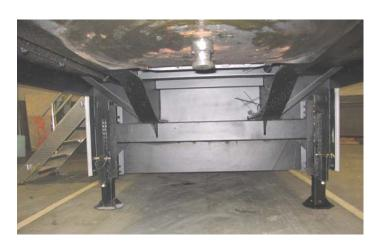
Figure 17: Front Stabilizing Legs and Auxiliary Support Legs
