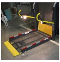
Wheel Chair Lift at floor level Figure 30: Wheel Chair Lift
